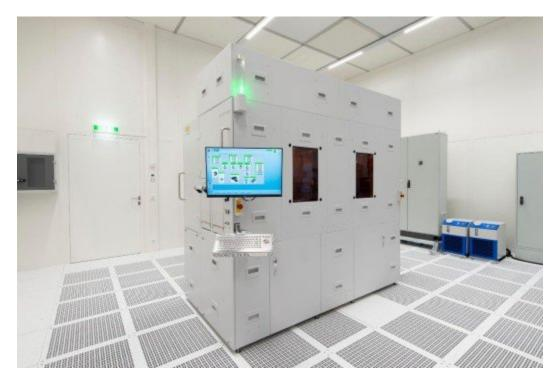
The EVG®150 automated resist processing system provides reliable and high-quality coating and developing processes in a universal platform that supports a variety of devices and applications, including advanced packaging, MEMS, radio frequency (RF), 3D sensing, power electronics, and photonics. Source: EV Group.
