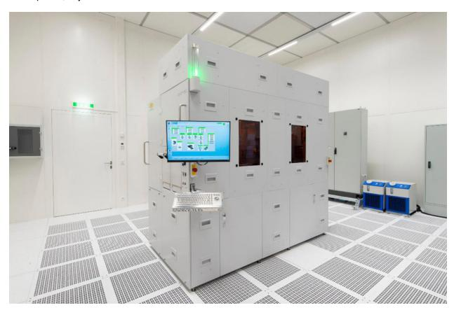
Picture: The EVG150 automated resist processing system.
