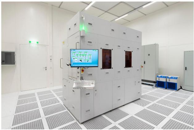
The EVG®150 automated resist processing system provides reliable and high-quality coating and developing processes in a universal platform that supports a variety of devices and applications, including advanced packaging, MEMS, radio frequency (RF), 3D sensing, power electronics, and photonics. Source: EV Group.
