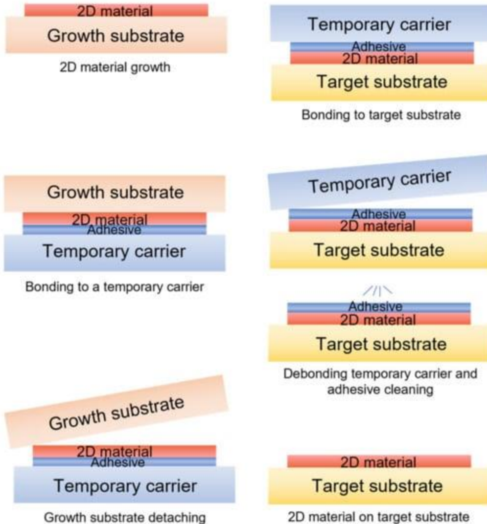
Figure 5. Two-dimensional layer transfer flow with TBDB technology.
