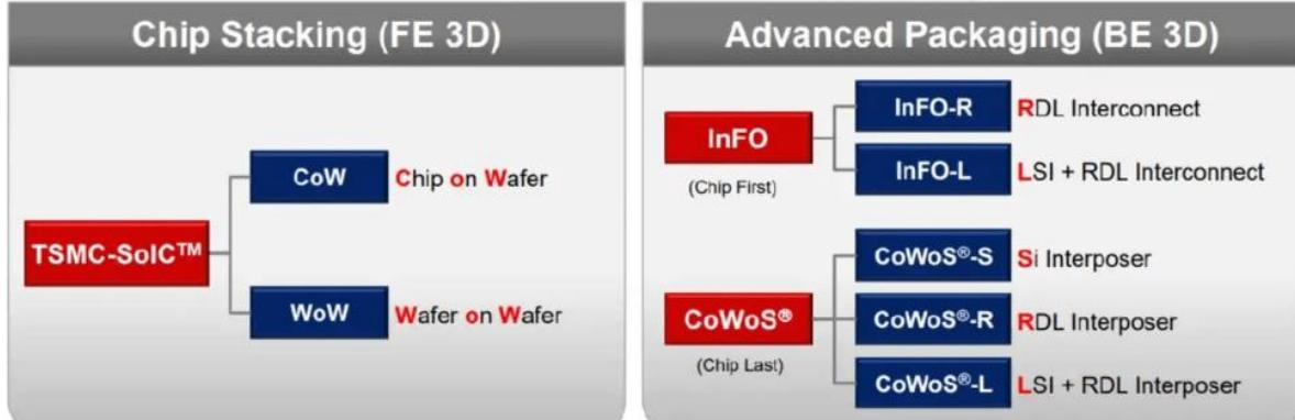
*SoIC: System on Integrated Chips*
