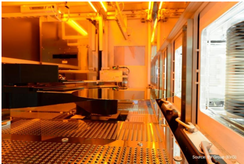
View inside the EVG®850 NanoCleave™ layer release system, with the pre-processing module bay and the mechanical release module in the background. Source: EV Group.
