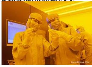
Process engineers examine a 200-mm wafer with metalenses replicated using a master manufactured by Toppan Photomask and a nanoimprint lithography process from EVG. The companies are collaborating to establish the process as an industry standard for photonics manufacturing. Courtesy of EV Group.
