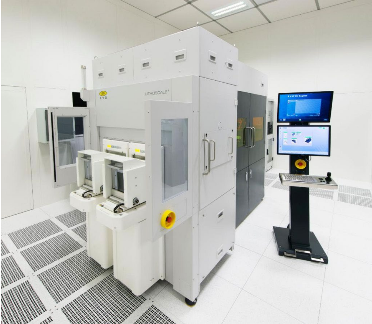
The LITHOSCALE maskless exposure lithography system from EV Group is one of several tools providing revolutionary process solutions to the Chip-let System Package Alliance (Hi-CHIP) led by ITRI. Source: EV Group.
