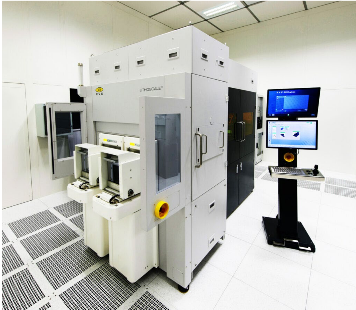
LITHOSCALE® maskless exposure lithography system from EV Group installed at ITRI Heterogeneous Chip Integration Trends
