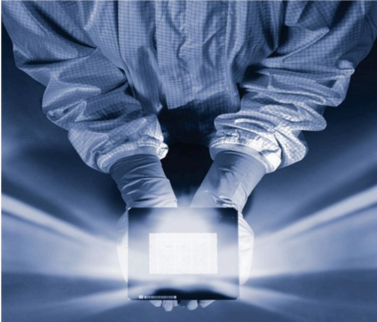
Toppan Photomask manufactures photomasks for the semiconductor industry like the one shown here. Nanoimprint lithography (NIL) masters are made using the same materials, technology and techniques. Source: Toppan Photomask.
