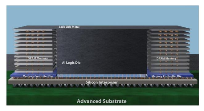
Heterogeneous integration brings new kinds of design and manufacturing flexibility to semiconductor and systems companies by allowing chips of various technologies, functions and sizes to be integrated in one package. Applied materials is combining its leadership in process technology and large-area substrates along with ecosystem collaborations to accelerate the industry's heterogeneous design and integration roadmaps.
