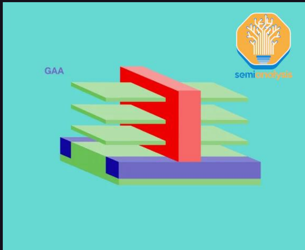
Cross section of the gate metal stack in GAA
