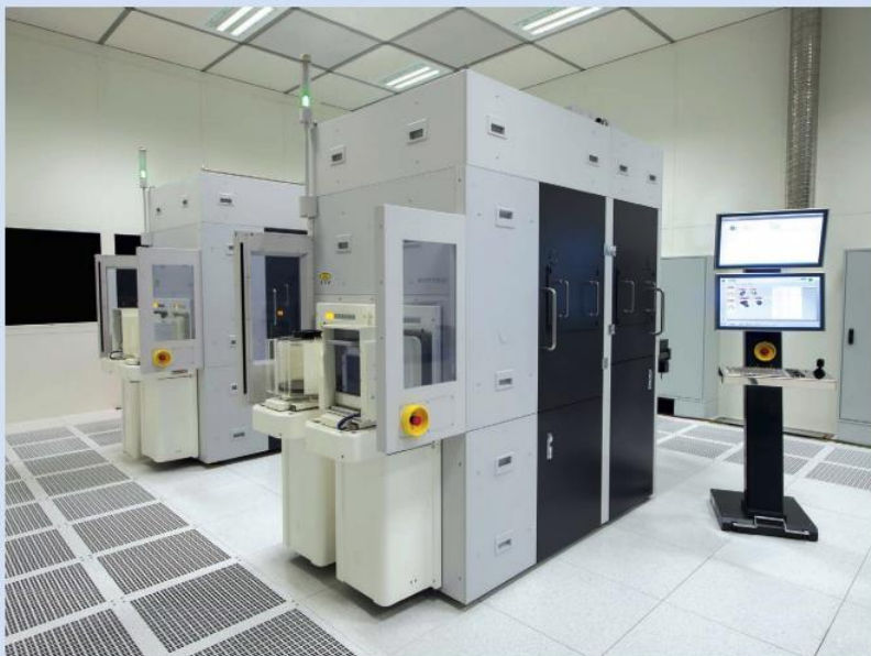
SAL has installed, among others, the UV-NIL system EVG7300 and complementary resist process systems in its R&D MicroFab in Villach, Austria. (Bild: EVG)
