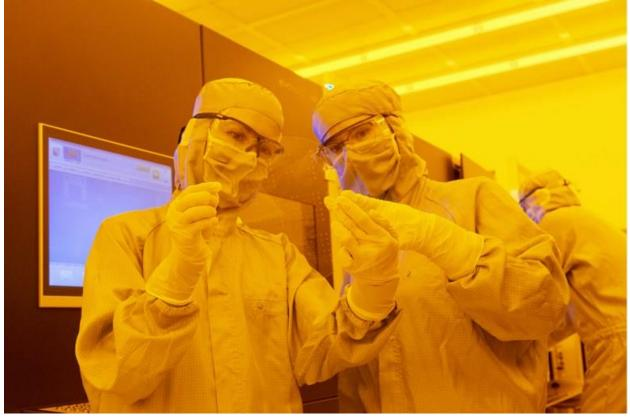
Process engineers at EV Group examine a 200mm wafer made using nanoimprint lithography technology. Image: EV Group
