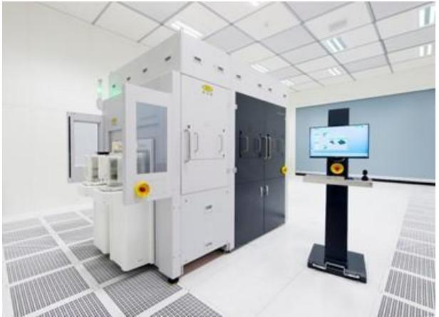
The EVG40 NT2 from the EV group provides breakthrough measurements for wafer- and die-level hybrid bonding and maskless lithography
