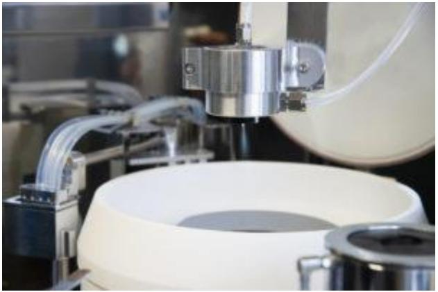
EV Group's proprietary OmniSpray® ultrasonic atomization technology provides unmatched process results when it comes to conformal coating of extreme topographies. Shown here is the OmniSpray module on an EVG120 automated resist processing system.
