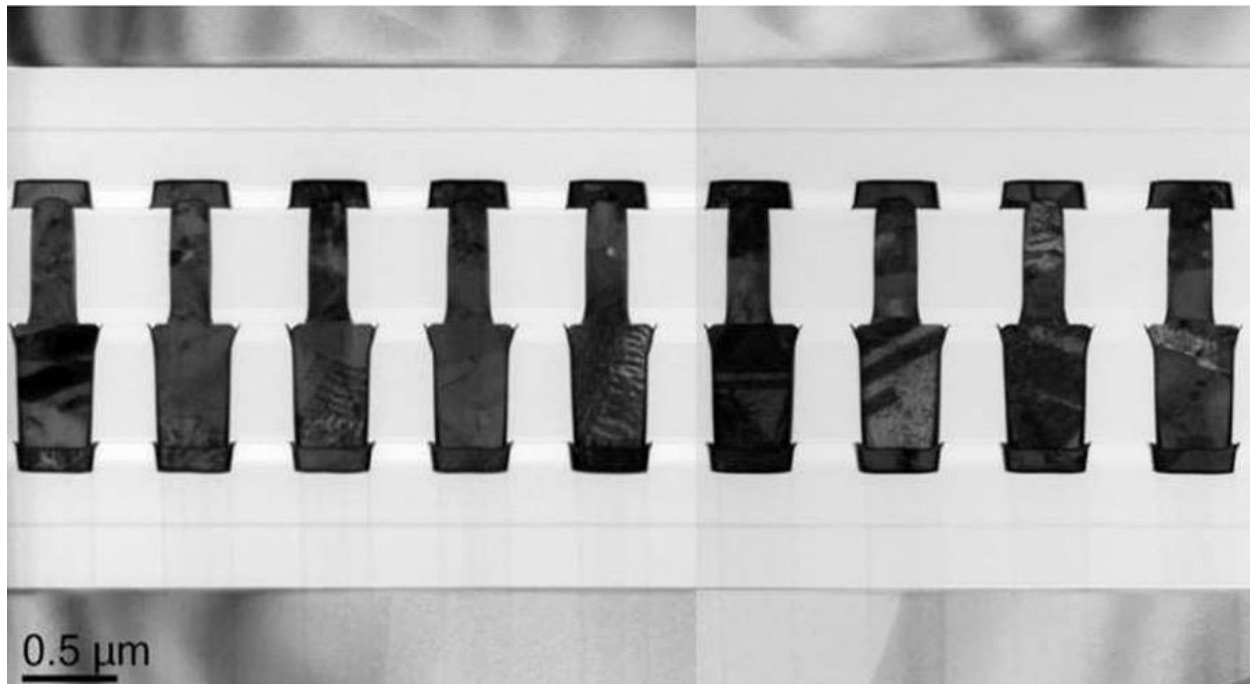
Fig. 3: Wafer-to-wafer hybrid bonding with 700nm metal pitch. Source: Imec, IEDM
