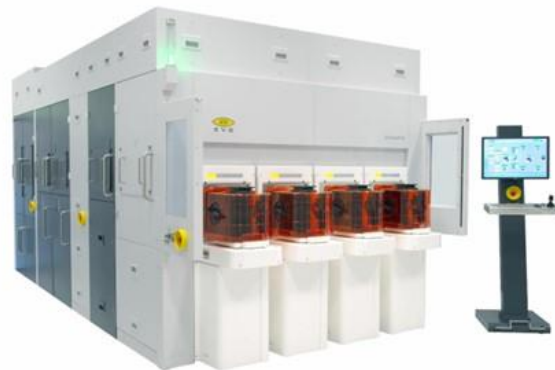
GEMINI®FB integrated fusion bonding system. Source: EV Group, 2022
