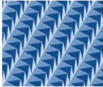
Fifty-micron-wide structures are replicated using EV Group's nanoimprint lithography solutions.
